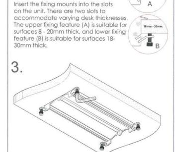
Screw the provided M8 x 20mm cap head fixing bolts through the fixing mounts until the unit is secure. Ensure
