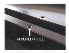
NOTE: Tapered holes must face up. As per image showing the difference between the two.
